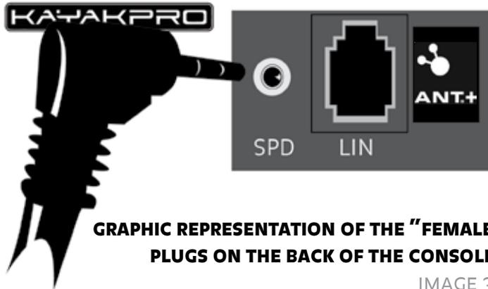
**GRAPHIC REPRESENTATION OF THE "FEMALE" PLUGS ON THE BACK OF THE CONSOLE**
