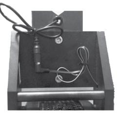
BACK OF THE FLYWHEEL IMAGE 1 The smaller 2 mm "male" plugged cable exiting from the middle of the frame is an extension on the cable connected at the flywheel end. This 2mm jack plugs into the back of the on-board console, the jack port marked "SPD." (See image 2 & 3 .)
