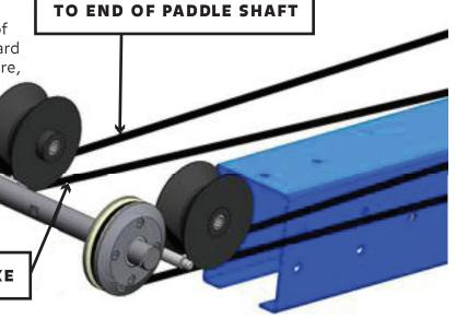
**STEP 7:** You will now assemble the paddle shaft (3 pieces). The piece without the ferrule installs in the middle. The other two pieces install on the outside with the screw pointed outward. For now, place the paddle shaft in its narrowest position, so it is as short as possible.
