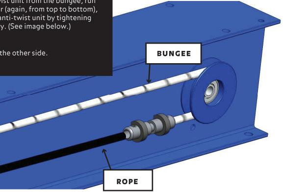
STEP 5: On one side of the Speedstroke, run the rope around the rollers at the front of the machine. near the Flywheel. Do this as pictured in the image below. The rope travels around the bottom of the silver front catch roller, exits the top of that roller, and then (under) the bottom of the black guide roller. The rope should exit toward the back of the machine (where the seat is), where, for now, you will leave it on the floor.
